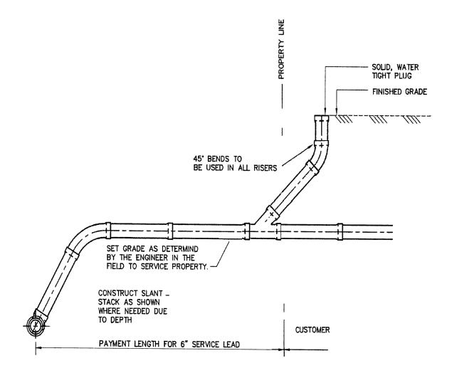
Lateral means that part of the sewer collection system extending from the sewer main to the owner's property line and located within the public right-of-way.
